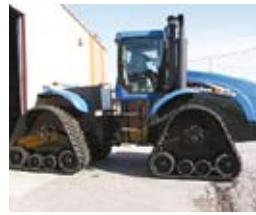
New Holland does not offer tracks as original equipment on its articulated 4WD Series TJ tractors, so the only solution is to fit tracks such as these ATI units
