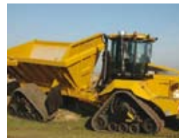
Bruko track units from Greccav on a Challenger TerraGator applications vehicle adapted for earthmoving operations
