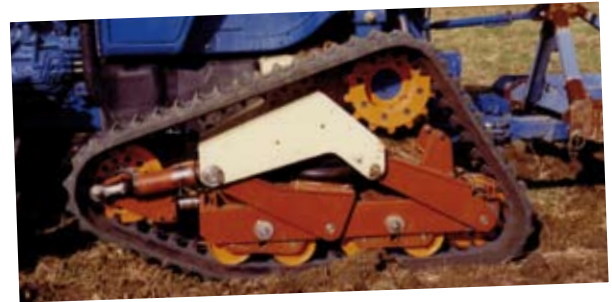
The pneumatic suspension system allows the track roller assembly to move up and down with the front idler moved in and out mechanically to maintain the correct traction belt tension
