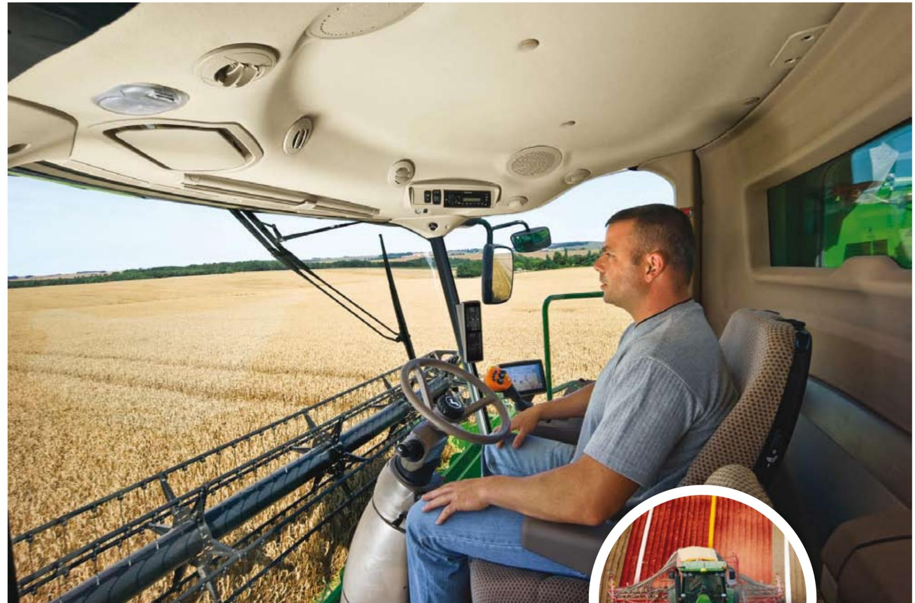
ABOVE AND RIGHT: John Deere's AutoTrac technology enables hands-free operation while enabling greater precision
