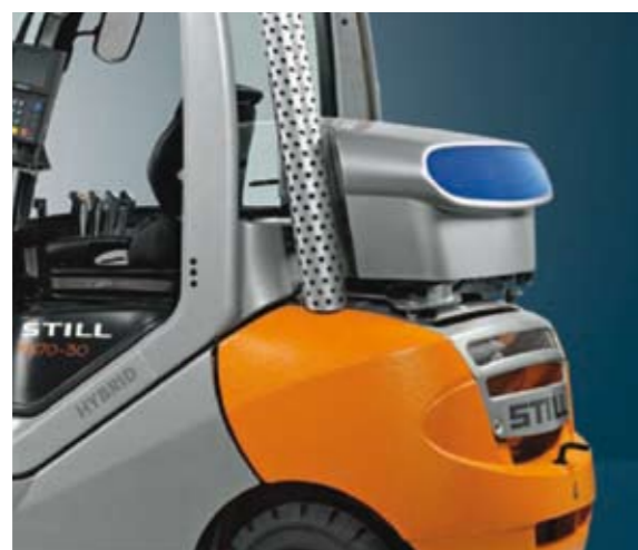
High-quality energy reservoirs are characterised by high energy and power density, cyclical life and perfect energy efficiency – pictured above is the bulkier stack of ultracapacitors seen on the 2008 prototype
